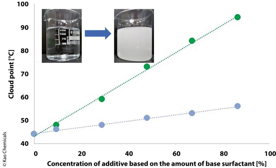
**Figure 2** > The cleaner formulation has a cloud point of 44 °C. This can be increased by adding an additive. As can be seen from the figure, Akypo has a significantly higher influence on the cloud point than a non-ionic surfactant (C1315 EO9).
