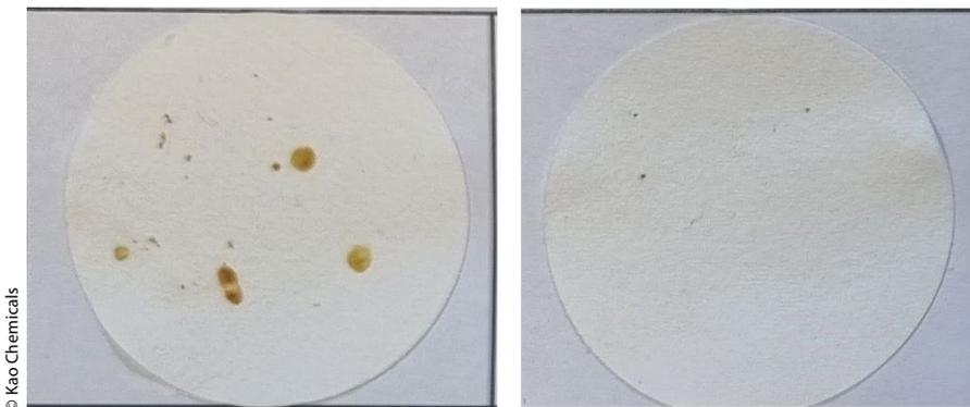
**Figure 3** > Corrosion protection behavior of different cleaner formulations according to DIN 51360-2. The right picture shows a combination of Akypo and an amine in the cleaner, which have formed a temporary corrosion protection. The left picture is from a cleaner based on non-ionic surfactants.
