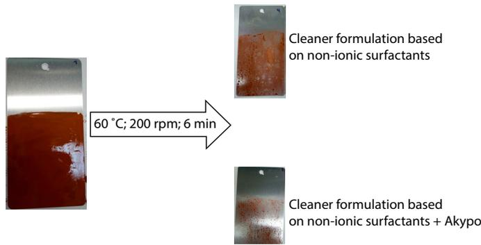
**Figure 4** > Increased cleaning efficiency of Akypo against dirt containing particles.
