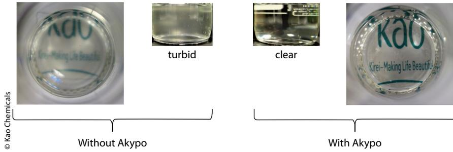
**Figure 1** > Stabilization of a defoamer in a cleaner concentrate, on the left unstable solution without Akypo, on the right stable solution with Akypo.
