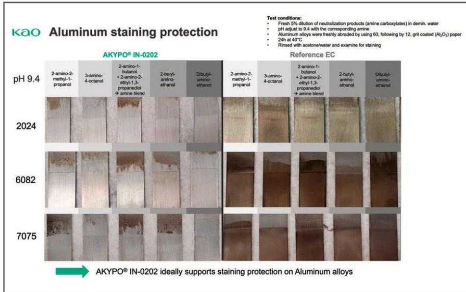
**Figure 3: Aluminum corrosion test with a 5% dilution of neutralized ether carboxylic acid with different amines to pH 9.4 in demineralized water. On the left AKYPO® IN-0202 ether carboxylic acid (EC) and on the right reference long-chain with high degree of ethoxylation EC. Staining is evaluated after 24 hours at 40°C.**
