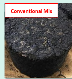
Samples after soaking in fuel for 24 hrs.
