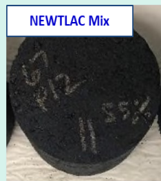
Samples after soaking in fuel for 24 hrs.
